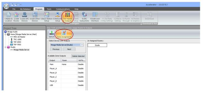
Tip (continued from step 5): In the Inputs tab, select the previously added monitor in the Select Device with Inputs section. Next, from the right pane, drag the MRX-20 Controller to the suitable Monitor input. For example, if you have connected the MRX-20 to monitor via HDMI, you can put the MRX-20 controller in the HDMI1 input of the monitor.
