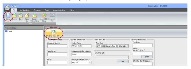
If iOS/Android devices are being used in the Total Control System, and the primary controller has not been configured previously with licensing information (purchased separately), click on **System Setup Codes** for entering the licenses. Configuring license with a controller is a one-time step, and can't be undone.
