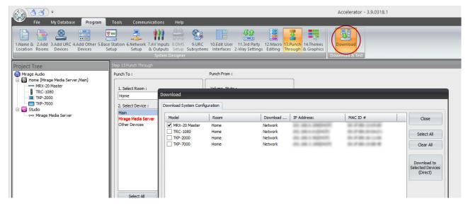
Tip: Occasionally, download fails to select clients like remotes and touchpanels. For instance, the panel drops wifi if screen is not on or if the remote is not charged. Touch the screen to switch it on, or place the remote on charger and try to download again.
