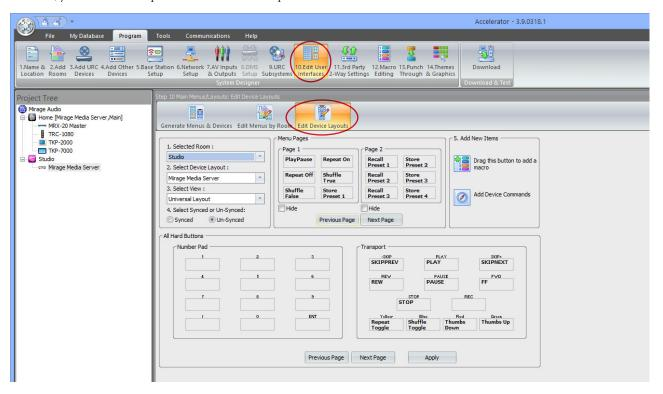
All Hard Buttons section shows all hard buttons and their currently assigned commands. Use Previous and Next page buttons to flip through all available hard buttons. Menu Pages section shows commands currently unassigned to any button. To change commands assigned to a hard button, simply drag a command to the new button. You can modify existing commands by dragging from one button to another, or assign new commands by dragging unassigned commands from Menu Pages section to an empty button.
