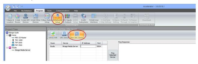
Click on the Ping Selected Device button to check if the MMS is reachable. The right pane displays the ping results. In case of any errors, please ensure the MMS is powered on and the correct IP address has been entered.
