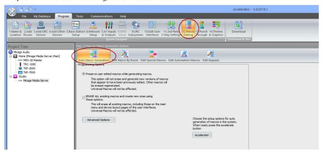
10. Go to Punch Through tab. This lets you control the functioning of hard buttons even when the Mirage Media Server module is not running. You can set it up to control Play, Pause, Skip Next and other functions for the MMS even if you're in the main menu.
